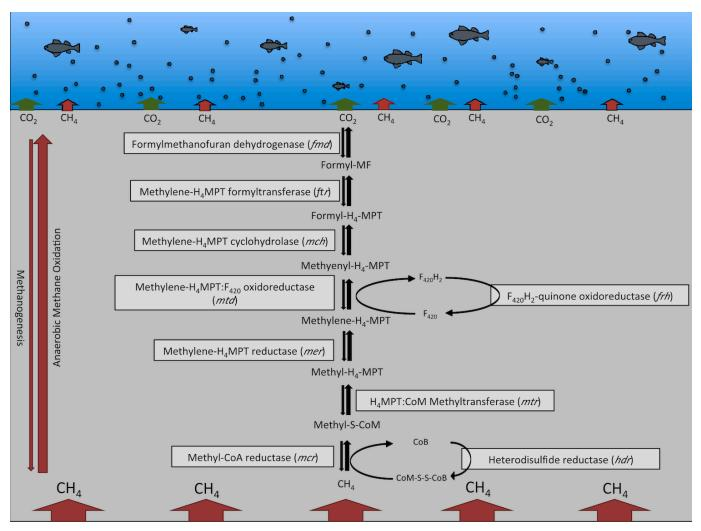
**Figure 1.** Anaerobic methane oxidation/methanogenesis in sediments of the Santa Barbara Channel. Proposed pathway based on the genes involved in AOM and methanogenesis identified in the metagenome from Santa Barbara Channel seep oil.
